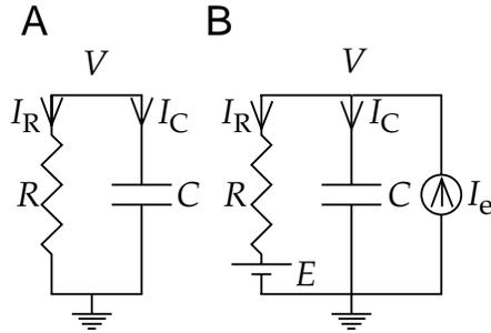
Figure 2: RC circuits. A) Current  $I_C = -I_R$  flows in the resistor-capacitor circuit as the stored charge is released. B) Simple passive membrane model including a potential  $E$  and current source  $I_e$ . As in figure 1, the lined triangles represent a ground or point of zero voltage.
