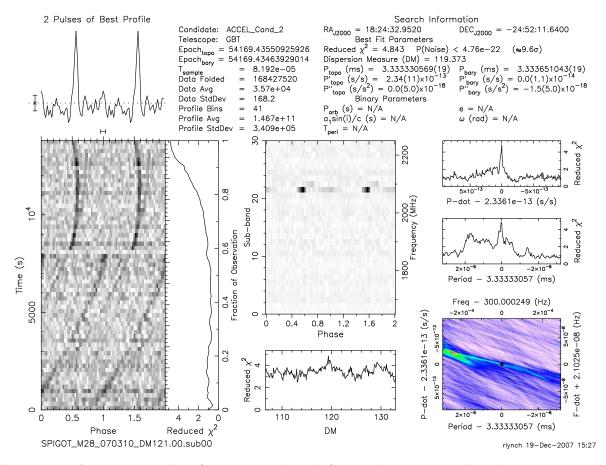
Fig. 12.— A prepfold plot of some RFI that drifts in phase. Notice the phase jump at 8000 seconds. There are other indications that this is RFI. The signal is narrow band, the DM curve is flat, and the Reduced  $\chi^2$  vs. Period curved doesn't peak at one period. Also, notice that the period is almost exactly  $3.\overline{3}$ , corresponding to a spin frequency of almost exactly 300 Hz. This is a suspiciously "convenient" period.
