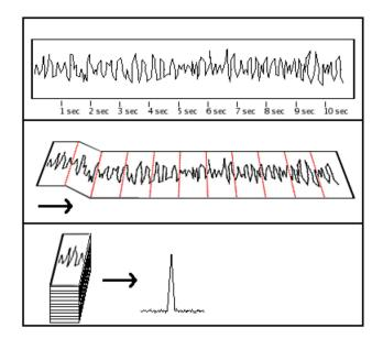
**Fig. 3.**— Here we illustrate the technique of folding. In the top panel, we place ticks every 1 second in our data. In the middle panel, we fold over at these tick marks. In the bottom panel, we add up the signal in each layer of our fold. In this way, we can find a weak pulsar that would otherwise be lost in the noise. However, we must know the period of the pulsar ahead of time. In this example, we used a period of one second.
