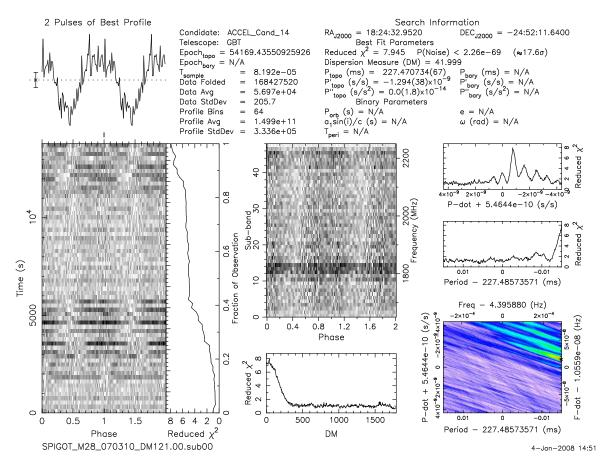
**Fig. 10.**— A **prepfold** plot of some broadband RFI that shows up at a variety of phases. This RFI is also transient. Another clue that this is RFI is that the DM curve peaks at zero.
