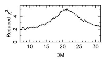
Fig. 7.— This panel shows the Dispersion Measure, or DM. The DM is a way of quantifying the number of electrons that the pulsar's signal must travel through to reach the Earth. The y-axis is the Reduced  $\chi^2$ . A real pulsar should have a peak value of Reduced  $\chi^2$  at a non-zero DM.
